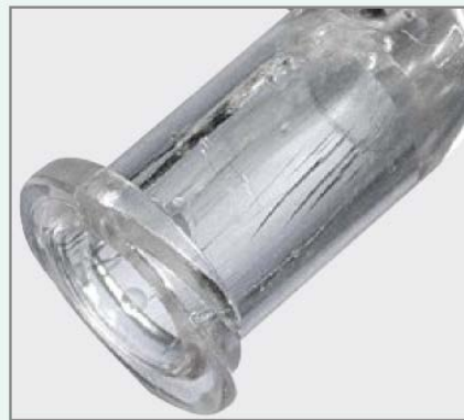
stress cracks due to material/drug incompatibility
